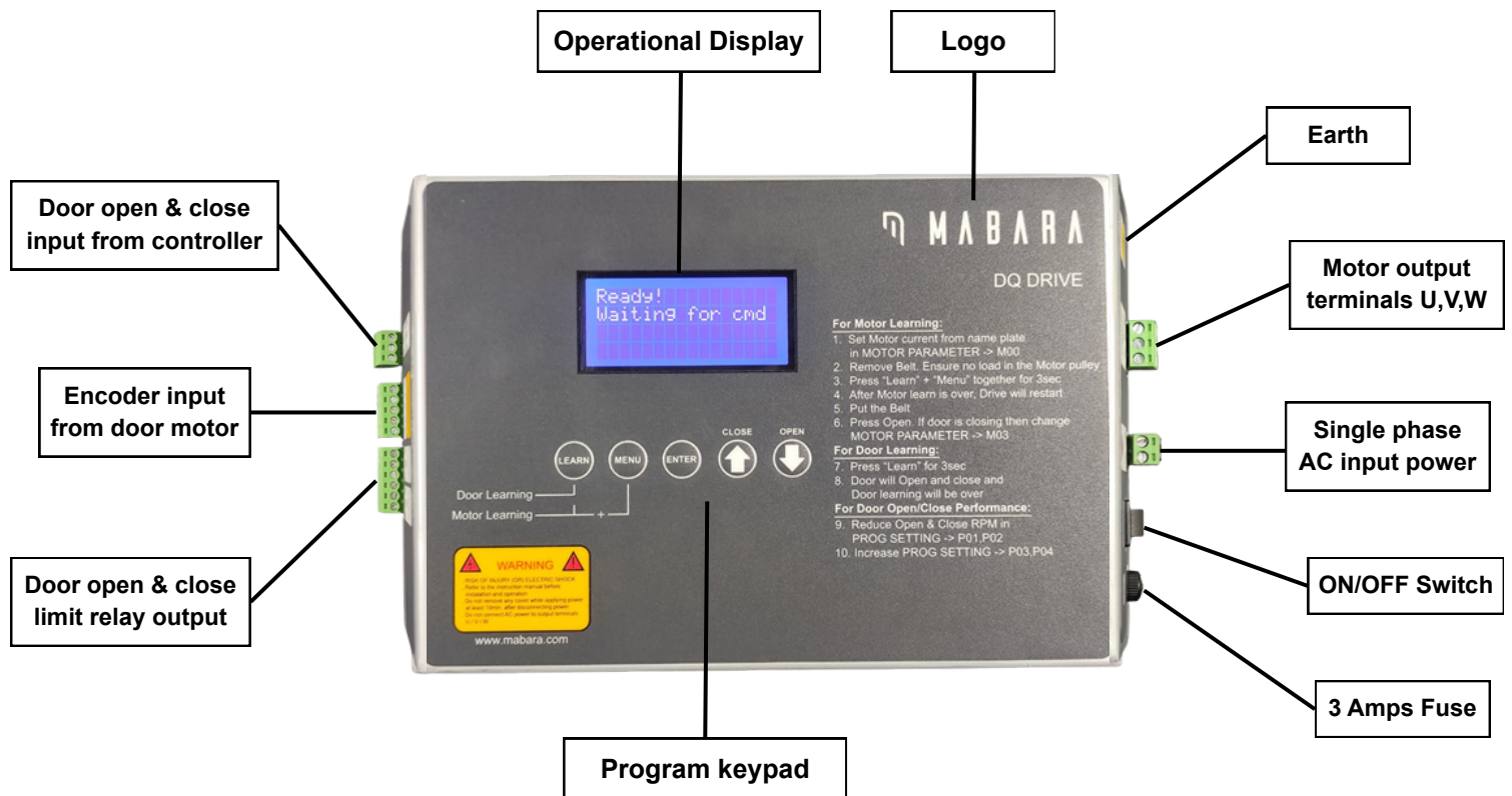
Figure 2-2 Structure of the MDDPM - DQ DRIVE
