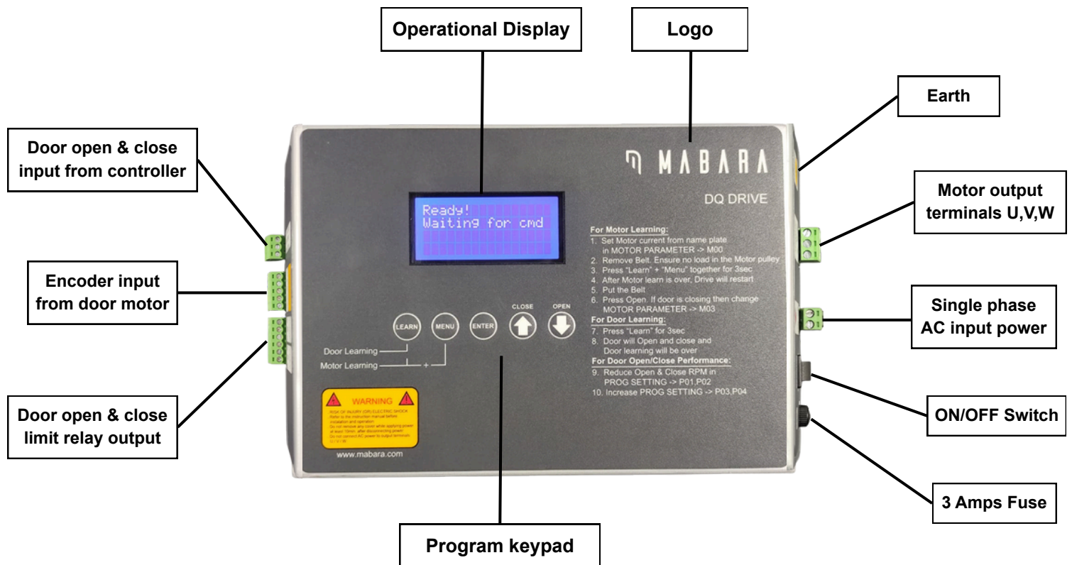
Figure 2-2 Structure of the MDDPM - DQ DRIVE
